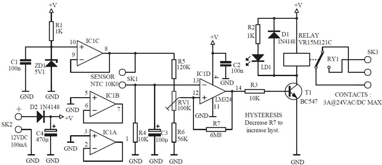
The central component is the comparator, which turns on the relay when the '+' side has less voltage than the '-' side. Let us simplify this to show the 'red' path for the '-' side and the 'blue' path for the '+' side being compared:
