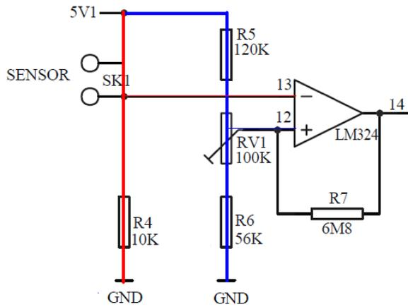
The + and – sides are simple resistor voltage dividers. The thermistor’s resistance changes as a function of its temperature, let us call it  $R_t$ .
